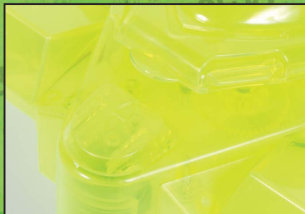
FIGURE 20. A sliding latch acts as a lock knob for holding the IR sensor holder against the program disk.
